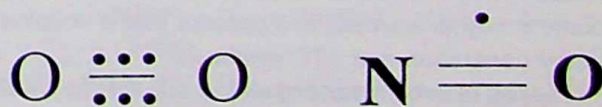
Fig. 1.— Electronic configuration of oxygen and nitric oxide molecules. The lines indicate full covalent bonds with a pair of electrons and the dots indicate single electrons. The oxygen molecule has two three-electron bonds and is a biradical. The nitric oxide molecule has one single unpaired electron and is a free radical.
